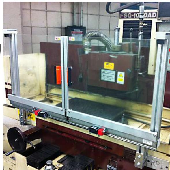
Equipped with two sliding doors on telescopic total-opening ball guides. Available with double anchorage system. Customized on request.
