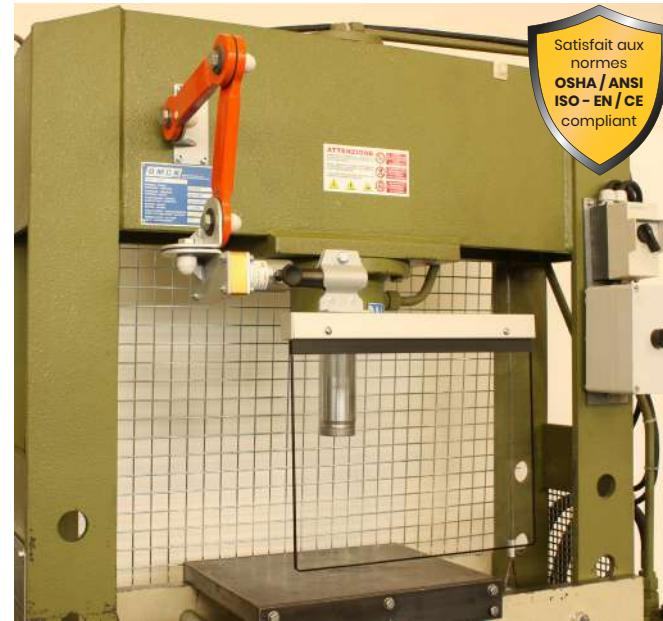
Universal articulated arms guard, with reversible opening direction. Practical and immediately adjustable. Designed for frequent changes of operation. Protects the operator from direct contact with dangerous parts frontally segregated by the shield. Frontally attachable to the machine. Equipped with wide «visibility» reversible opening shield: vertical, horizontal, left or right, with position-release knob. Equipped with a safety microswitch.
