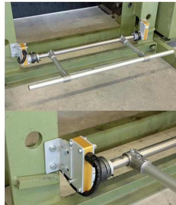
*Solid and versatile device, to be used as Stop-Start - Emergency system. Operated with arms or feet. Also customized on request.*
