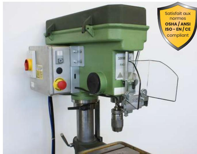
New safety shield offered with a double fixing system, supported by adjustable hexagonal arms. Equipped with a microswitch integrated in the rotation hinge.
