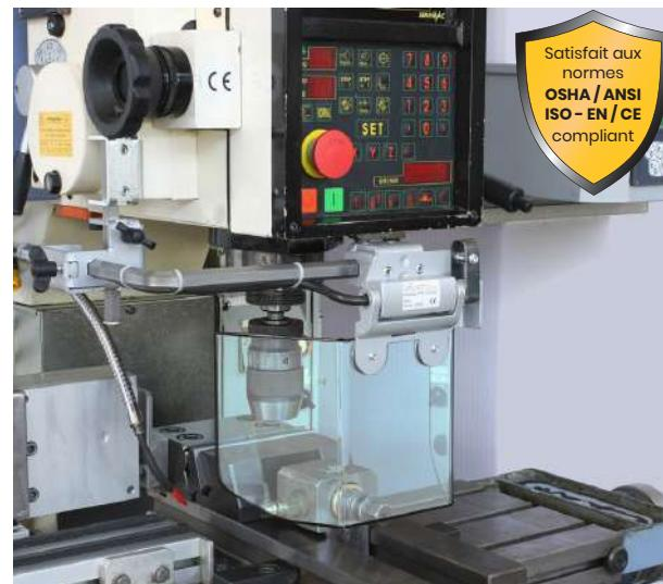
Exclusive safety guard supported by adjustable hexagonal arms. Equipped with vertical opening shield, with microswitch integrated in the rotation hinge.
