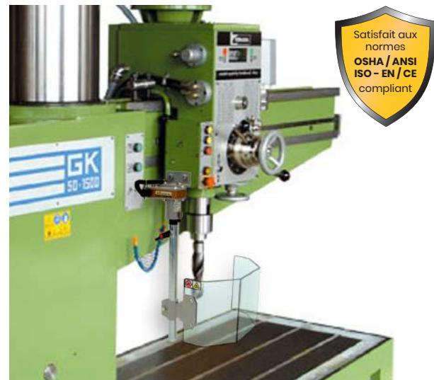
Safety guard equipped with vertical adjustment of the shield with a telescopic arm system. Suitable to be used on large-dimension drills and radial drills.
